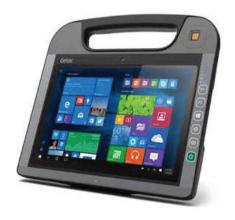
The Getac RX10 is powered by an Intel Core M-5Y10c (0.8GHz) or M-5Y71 vPro (1.2GHz) processor. The RX10 can be configured with tri pass-through antenna ports, allowing users to simultaneously connect high-gain GPS, WWAN and WLAN roof-mounted antenna for expanded signal range.
